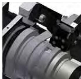
Magnetic encoder and brake on C-axis
